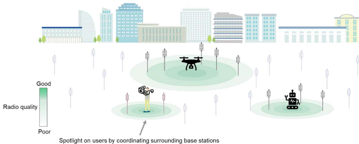
Figure 2-2 The concept of user-centric radio quality assurance.
